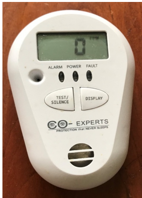
Carbon Monoxide Monitor
