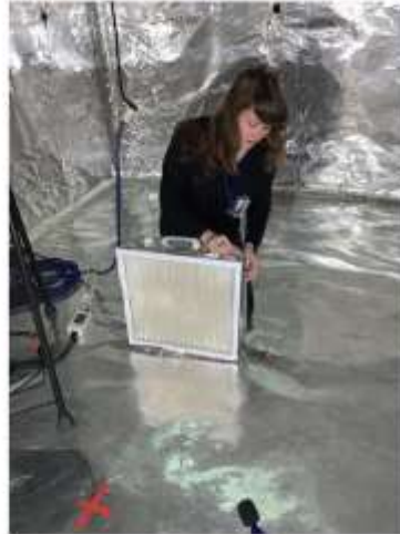
EPA researcher, Heidi Vreeland, testing a DIY air cleaner.
